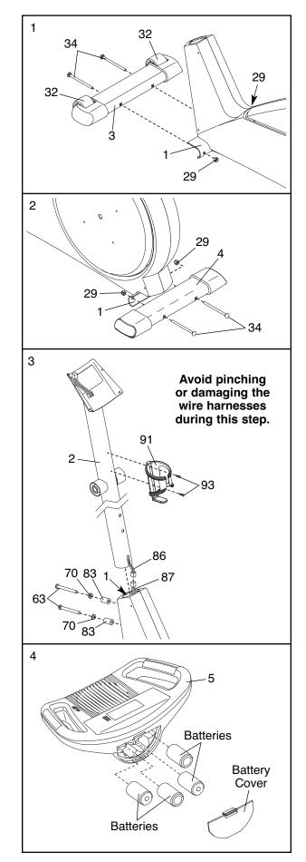
While another person holds the Console (5) in the position shown, connect the wire harness on the Console to the Upper Wire Harness (86). Insert the excess wire harness into the Upright (2). Next, attach the Console to the Upright with four M4 x 16mm Screws (66). Be careful to avoid pinching the wire harnesses.
